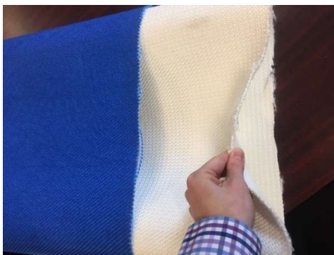
Figure 2: 12" woven hose, with inner woven layer (white) and outer woven layer (blue)
