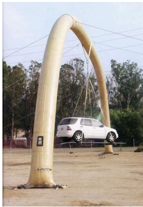
Figure 1: Inflatable support structure, strong enough to support substantial loads, such as an SUV
