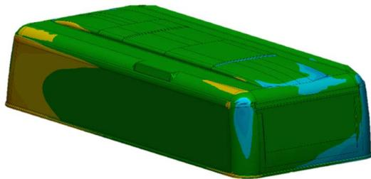
**Figure 5:** Deviation map of model vs. scan. Green areas indicate deviation of less than 6.35mm (1/4"), within tolerance
