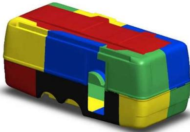
**Figure 4:** The trailer was segmented into 17 parts for Phase I.
