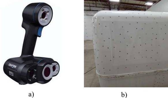
**Figure 2:** a) GoScan 3D scanner from CREAFORM, b) trailer segment ready for scanning, marked with positioning targets to maximize accuracy
