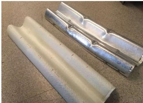
**Figure 1:** Illustration of roadway guardrails; the standard, stainless steel variant (top-right, after being subjected to three-point bend testing) and the fiberglass-PP variant (bottom-left)
