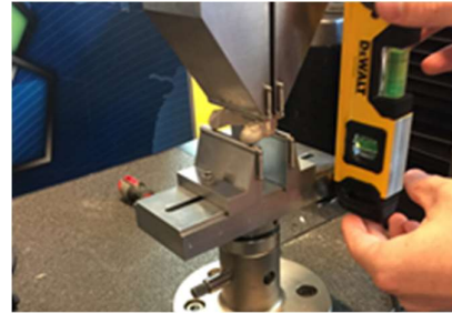
Figure 2: Mechanical testing set-up for the 4-point loading of dental implant samples, in an Instron 5969 load frame using an ASTM D790 fixture.
