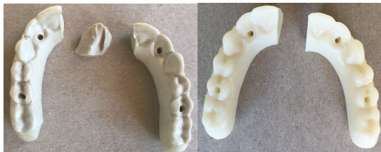
Figure 4: Failure modes of (left) PEEK and (right) PMMA. The PEEK experienced a significantly higher failure load than the PMMA, likely in part due to the manufacturing process used.
