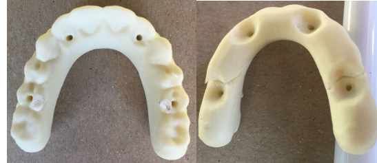
Figure 5: FRC sample shown in (left) top and (right) back-face orientations. The crack did not render the sample fully failed, with fibres bridged between the fracture planes for residual strength.
