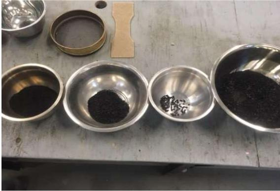
Fig. 2. Biochar particles with different sizes separated through sieving process.
