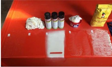
**Figure 4:** Application of wax, developer paint, flour and other materials to the GFRP surface.
