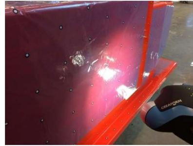
**Figure 5:** GFRP surface being scanned in-situ.
