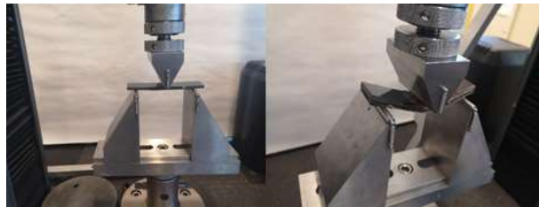
Figure 5. Three point bending using an Instron
